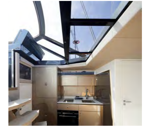
Sliding glass roof over Galley & Dining
